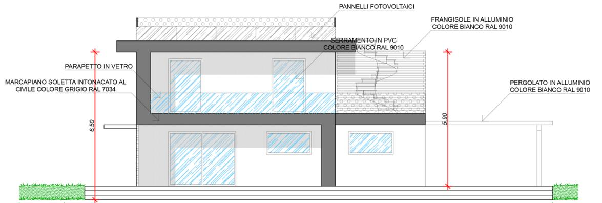
**PROSPETTO EST STATO DI PROGETTO SCALA 1:100**
