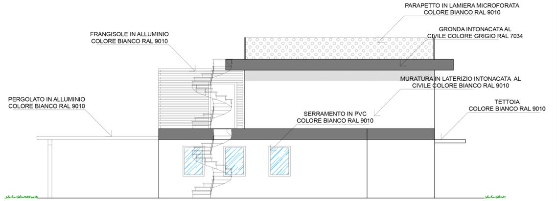
**PROSPETTO OVEST STATO DI PROGETTO SCALA 1:100**
